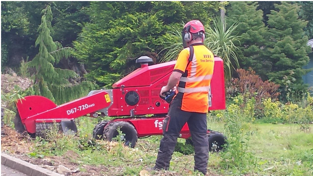
Stump Grinder -this greatly reduces work time on completing jobs in a shorter timeframe
